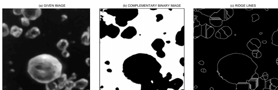
Fig. 1. Crystallographic image processing presenting (a) microscopic image, (b) its binary representation, and (c) ridge lines detection resulting from its watershed transform
