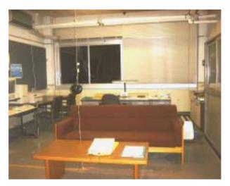
Figure 1: Insight view of reference room with installed globe (Vernon) thermometer in the interior's center
