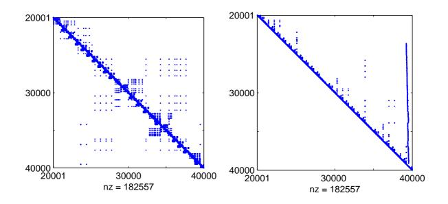
Figure 4: Tarjan's permuting (right) of a diagonal  $20\,000 \times 20\,000$  submatrix (left) of the SB-matrix.
