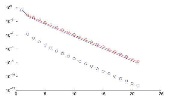
Figure 6: Graphical plot of the errors for Test 2 -  $20000 \times 20000$  submatrix of S-matrix, s = 1, t = 5, n = 100. Red line - power method, blue line - IAD method. Red circles - power method after Tarjan's reordering, blue circles - IAD method after Tarjan's reordering.
