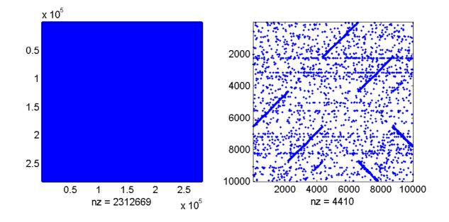
Figure 1: Sparsity structure of S-matrix. The whole matrix (resolution is not fine enough) and a diagonal submatrix with indices  $1 - 10\,000$ .
