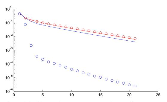
Figure 5: Graphical plot of the errors for Test 1 -  $20000 \times 20000$  submatrix of S-matrix, s = t = 1, n = 100. Red line - power method, blue line - IAD method. Red circles - power method after Tarjan's reordering, blue circles - IAD method after Tarjan's reordering.
