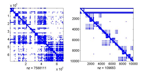
Figure 2: Sparsity structure of SB-matrix. The whole matrix and a diagonal submatrix with indices  $1 - 10\,000$ .
