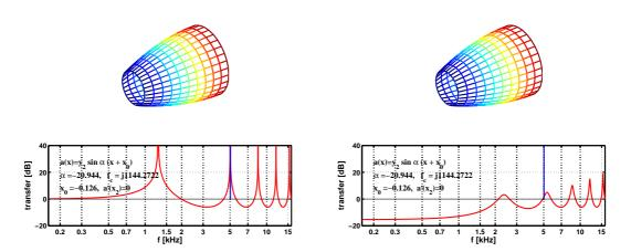
Figure 3: A sine waveguide – with rigid closure (left), with radiation impedance termination (right).
