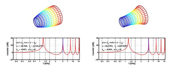
Figure 5: A cosine (left) and a catenoid (right) waveguide
