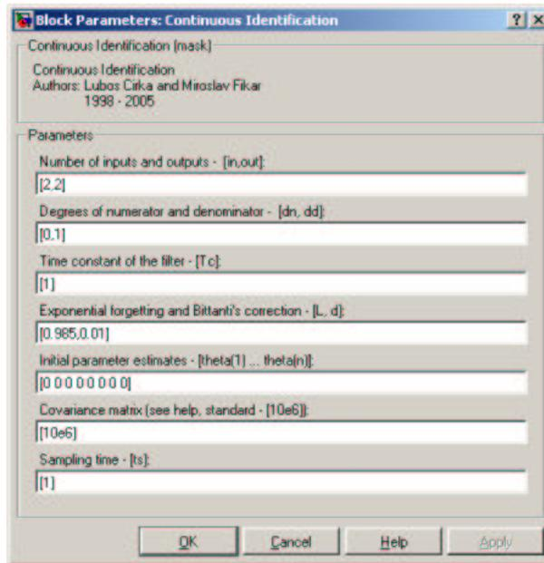
Figure 3: Block Parameters: Continuous Identification
