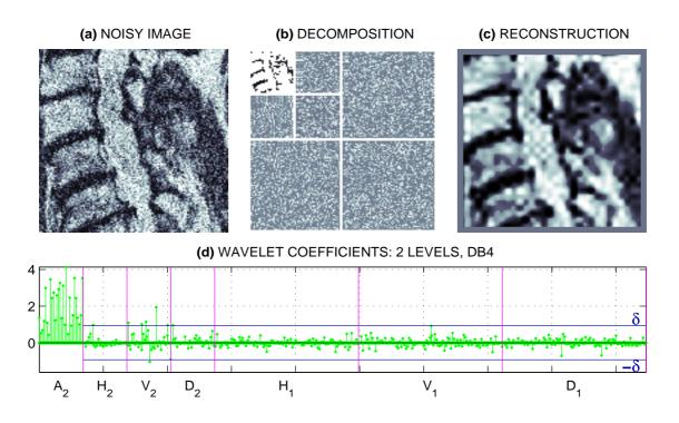
Figure 4: MR image de-noising by thresholding of the wavelet detail coefficients up to the second level presenting (a) MR image with the additional random noise, (b) decomposition up to the second level using the db4 wavelet function, (c) image reconstruction after the thresholding of wavelet coefficients, and (d) wavelet coefficients of the noisy image and the estimated threshold level  $\delta$
