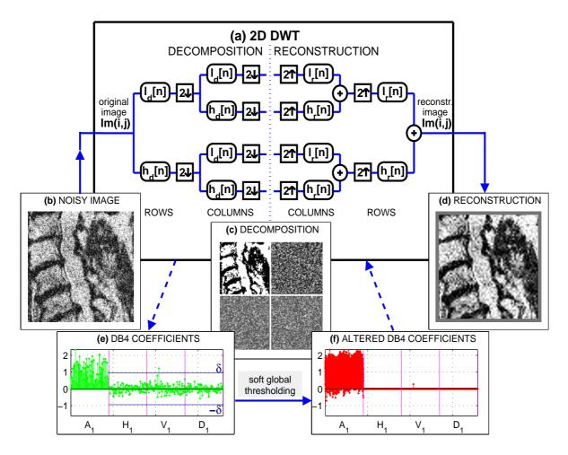
Figure 3: MR image enhancement by thresholding of the wavelet decomposition coefficients presenting (a) one-dimensional wavelet subband coding scheme, (b) noisy MR image, (c) first level decomposition using the *db4* wavelet function, (d) reconstructed and interpolated image, (e) absolute *db4* decomposition coefficients, and (f) thresholded decomposition coefficients used for image reconstruction
