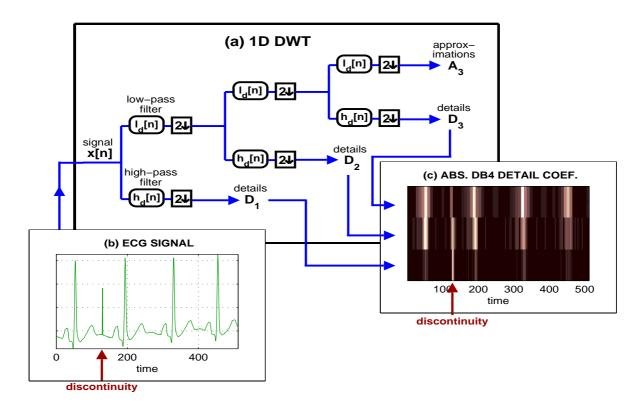
Figure 1: Discontinuity detection in the ECG signal applying wavelet analysis and presenting (a) one-dimensional wavelet subband coding scheme, (b) ECG signal with a discontinuity, and (c) absolute detail decomposition coefficients using the *db*4 wavelet function
