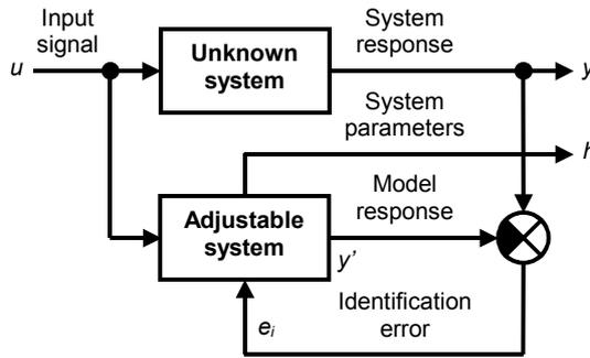
Figure 1: Direct system identification
