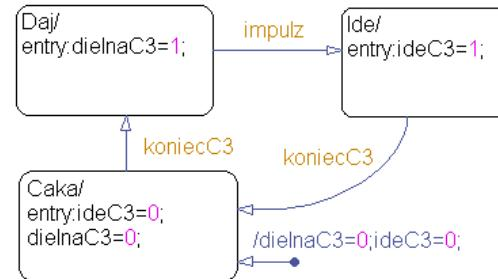
Figure 4: State representation of the conveyor C3
