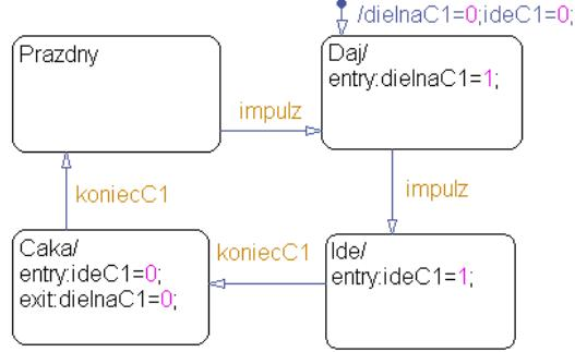
Figure 2: State representation of the conveyor C1
