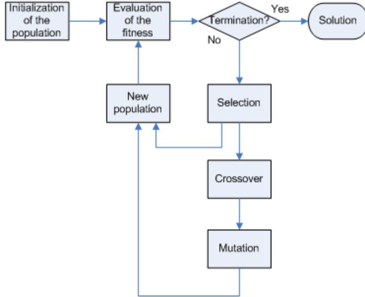
Figure 7: Block scheme of the genetic algorithm
