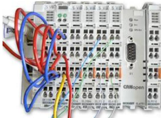
Figure 8: Connection of the slave devices on the strip, there is also a CANOpen extension module present
