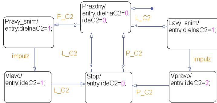
Figure 3: State representation of the conveyor C2
