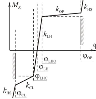
Figure 3. Schema of nonlinear spring (LH – limp home, CL – throttle closed, OP – throttle opened)
