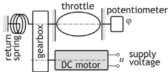
Figure 2. Schema of throttle
