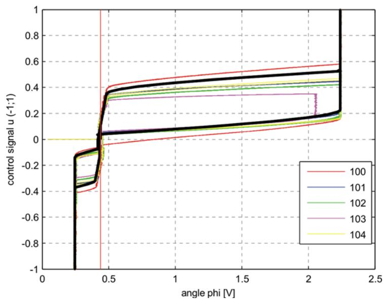
Figure 6. Static  $\varphi - u$  characteristic measured and filtered (colored) and identified model (black)
