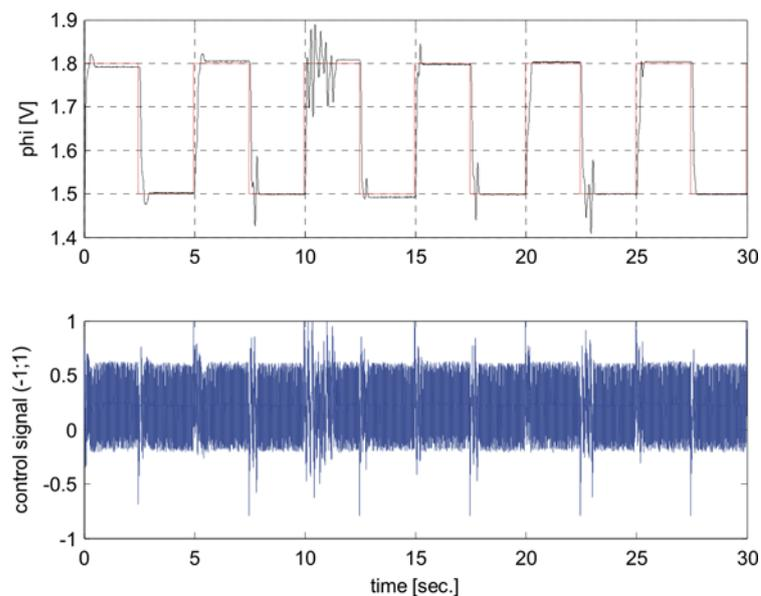
Figure 11. Response of controlled system with no friction compensation
