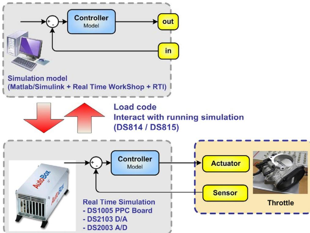
Figure 8: Principal schematic of RCP
