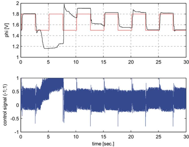
Figure 12. Response of controlled system after the manual disturbance of valve position
