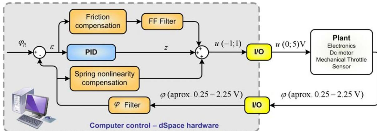
Figure 9. Schema of nonlinear controller
