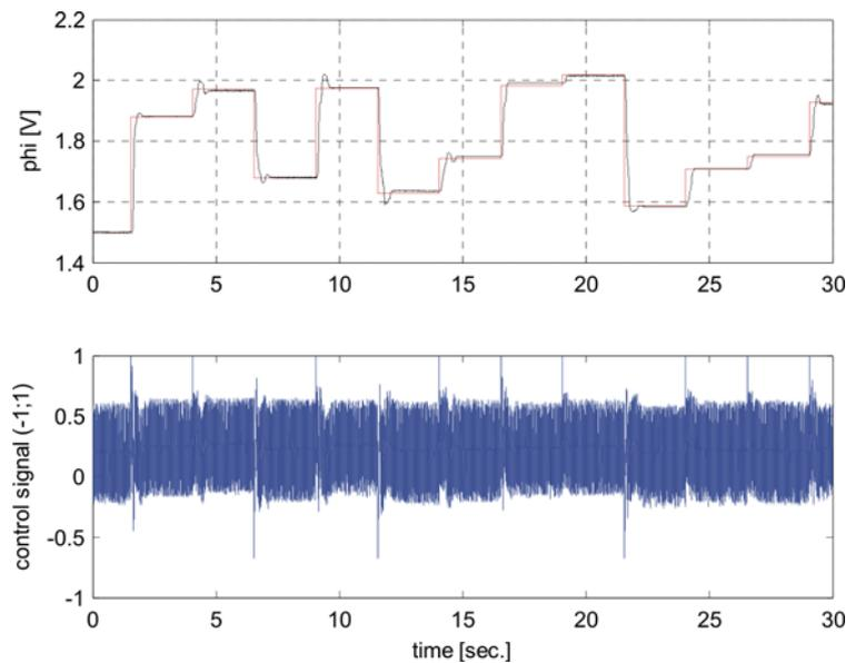
Figure 10. Response of controlled system to random desired step values
