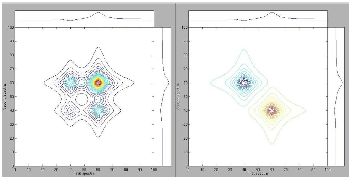
Figure 9: Synchronous and asynchronous 2D spectra of 2 growing ROA/VCD Lorentzian peaks.
