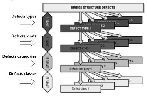
Figure 1: Hierarchical classification of railway bridge defects
