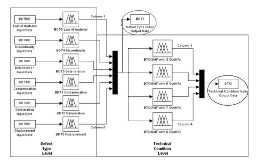
Figure 3: Architecture of the proposed two-level fuzzy system for the technical condition evaluation of mass concrete and/or stone bridge substructure
