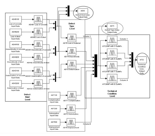
Figure 2: Architecture of the proposed three-level fuzzy system for the technical condition evaluation of steel-concrete bridge superstructure
