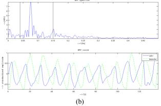
Fig. 3. Power spectrum for (a) uncontrolled respiration and (b) respiration during deep breathing test.
