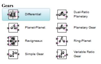
The Gears library contains blocks that represent simple and complex gears, driveline elements that couple distinct driveline axes and constrain their relative motions. The Gear blocks range from simple two-wheel gear couplings with fixed and variable gear ratios, to complex multiwheel and multiaxis gears such as planetary and differential gears.
