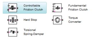
The Dynamic Elements library contains blocks that model such critical drivetrain components as clutches, torque converters, damped springs, and stops. Dynamic elements generate internal driveline torques. The blocks of this library serve as suggestions for developing variant or entirely new models to simulate the same components. Look under the block mask, break the block's library link before modifying it, and create your own version.
