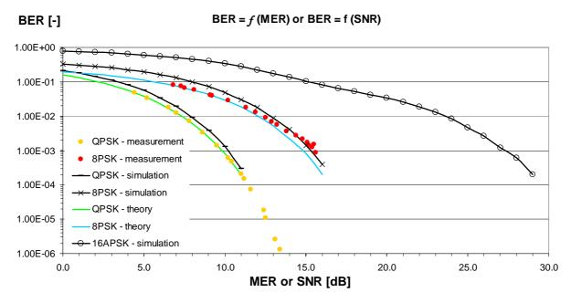
Figure 5: Characteristics of the *BER* (Bit Error Rate) in dependence on *MER* (Modulation Error Rate) in case of the measurements or *SNR* (Signal-to-Noise Ratio) in case of the simulation in Matlab.
