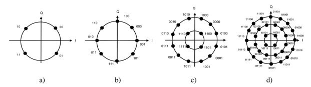
Figure 1: Constellation diagrams of digital modulations a) QPSK, b) 8PSK, c) 16APSK, d) 32APSK.
