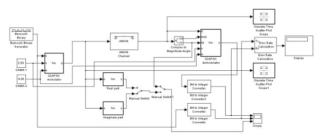
Figure 3: Model used for finding out dependence of *BER* (Bit Error Rate) on *SNR* (Signal-to-Noise Ratio) and constellation analysis assignment for 16APSK and 32APSK.
