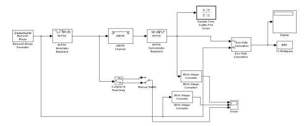
Figure 2: Model used for finding out dependence of *BER* (Bit Error Rate) on *SNR* (Signal-to-Noise Ratio) and constellation analysis assignment for QPSK and 8PSK.
