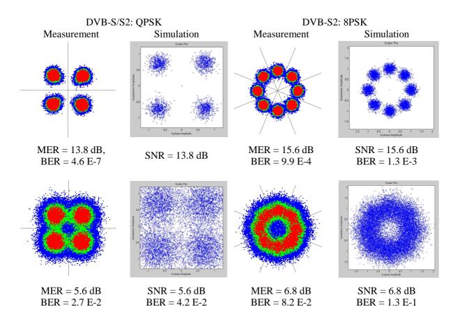
Figure 4: Constellation diagrams of modulations used for broadcasting in DVB-S/S2 systems with two values of *MER / SNR* measured and simulated in Matlab.
