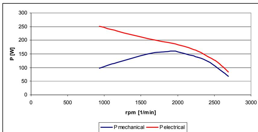
Figure 11: Waveform of electrical power of DC/AC/AC converter and mechanical power from 2-phase ASM motor
