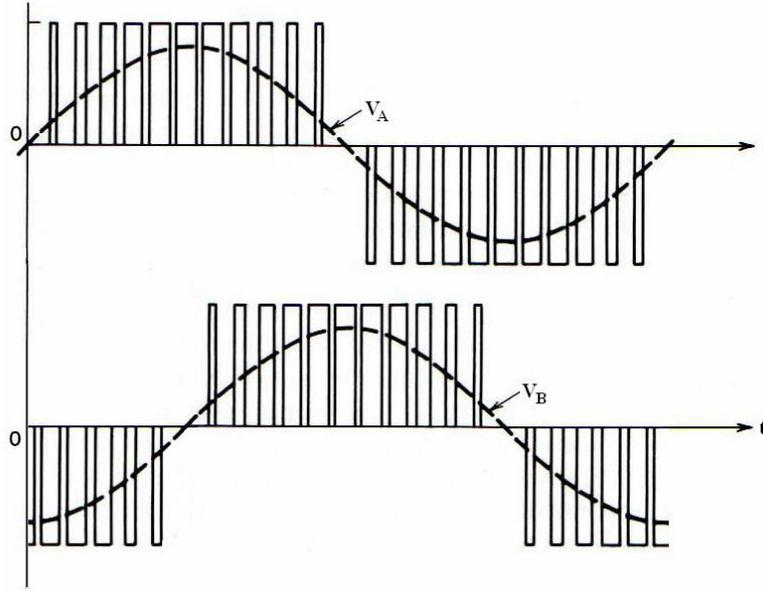
Figure 5: Voltages waveforms of unipolar PWM
