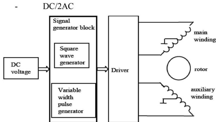
Figure 1: Block diagram for single-stage two-phase motor drive system supplied from DC source [1]
