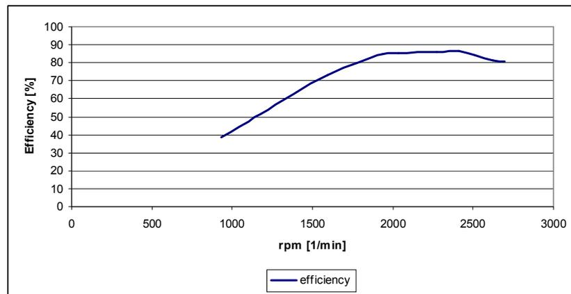
Figure 12: Efficiency waveform of DC/AC/AC converter and 2-phase ASM motor system
