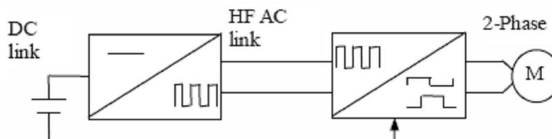
Figure 2: Principle block diagram of 2-stage DC/AC/AC converter (without HF transformer) and with 2-phase second stage [2]
