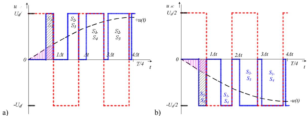
Figure 6. Switching strategy of half bridge converter for a) positive and b) negative half period of operation
