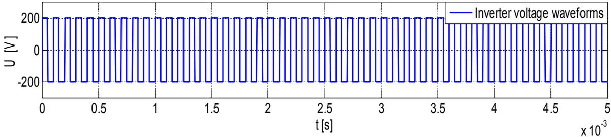
Figure 4: Voltage waveforms of AC HF interlink (first stage)
