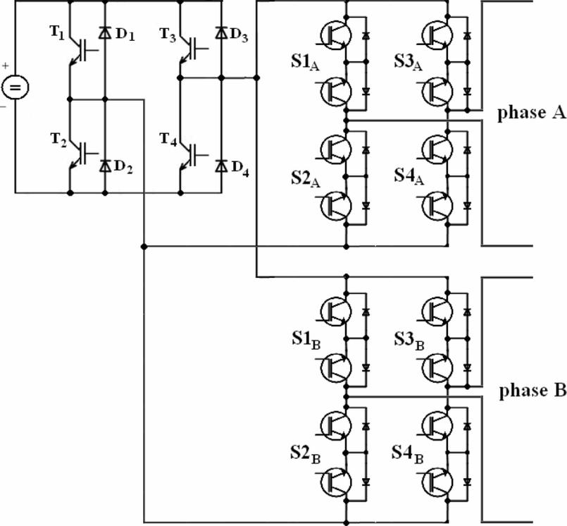
Figure 3: Two-stage two-phase DC-AC-AC converter
