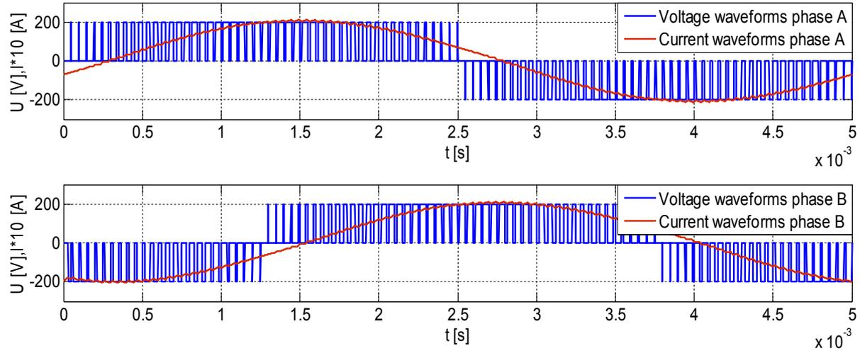
Figure 7: Voltage and current waveforms of matrix converter
