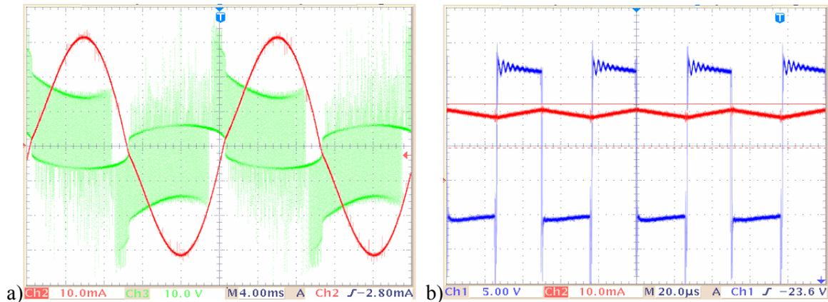
Figure 10: a) Output voltage (switched waveform) and current (continuous waveform) of DC/AC/AC converter and b) it's detail view ( $f_{sw}=20\text{kHz}$ ,  $f_{out}=50\text{Hz}$ ) [7]
