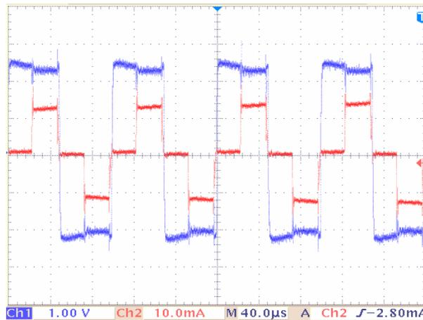
Figure 9: Waveform of voltage and current in AC HF interlink ( $f_{sw}=20\text{kHz}$ ) [7]
