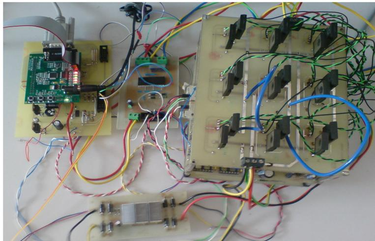
Figure 8: Physical model of single-phase inverter and matrix converter [7]
