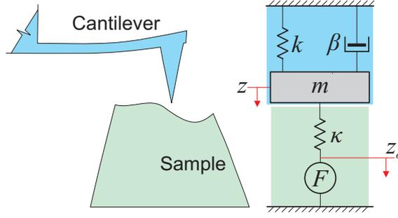
Figure 1: The model of the system (right) and corresponding elements of the Atomic Force Microscopy, the major branch of the Scanning Probe Microscopy (left).
