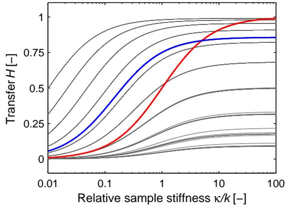
Figure 3: Effect of the feedback on the magnitude of the frequency response at given pass-band frequency versus  $\kappa/k$  ratio is depicted below. Blue curve represents case with feedback  $P = 6$ ,  $I = 4$ . Gray lines represent cases with feedback with parameters logarithmically distributed between 0.1 and 100. Red curve shows case without feedback.
