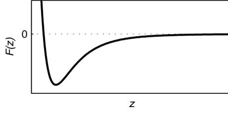
Figure 2: The Lennard-Jones force versus sample-probe distance,  $z$ . Arbitrary units.
