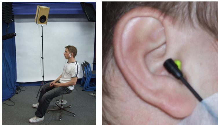
Figure 2: Measuring of HRTF – a) whole measuring set b) detail on microphone attachment.
