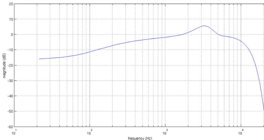
Figure 1: Response of the FIR filter designed according to the ITU norm [7].
