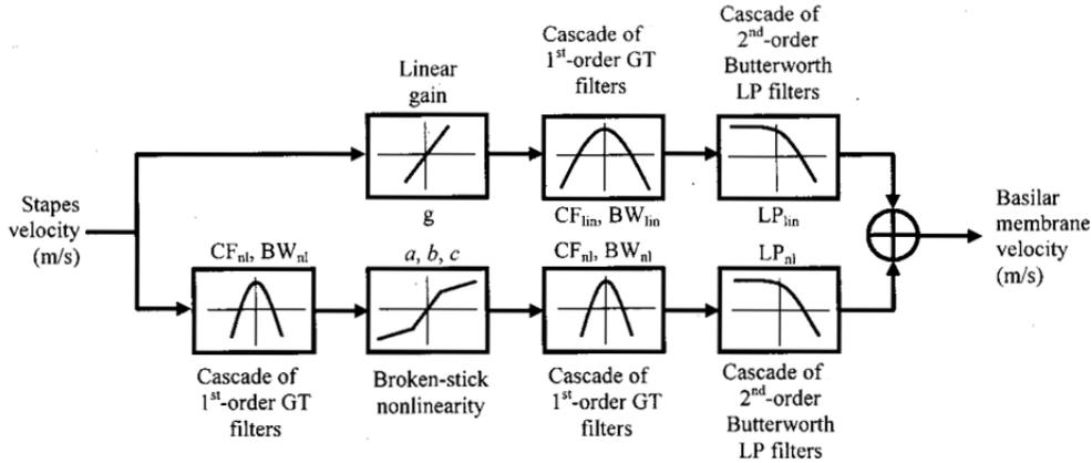
Figure 2: Diagram of the dual resonance nonlinear filter. The filter has two parts. The first one is linear and the second one nonlinear. Nonlinear stage is dominant for the signal frequencies close to the filter’s center frequency and for the low level signals [9].
