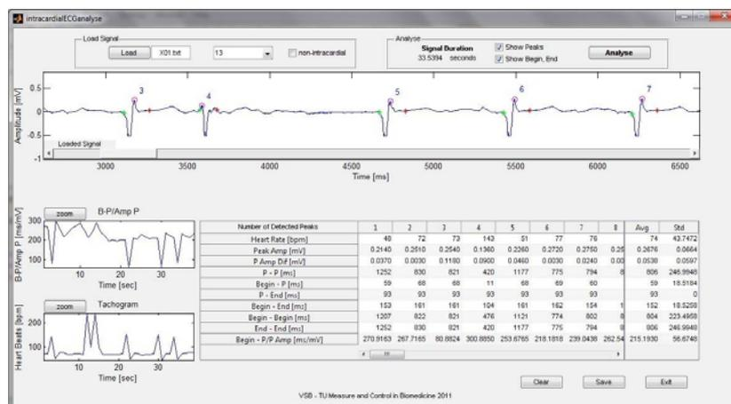
Figure 8: Sample intracardial ECG analysis running the program, after loading and signal
