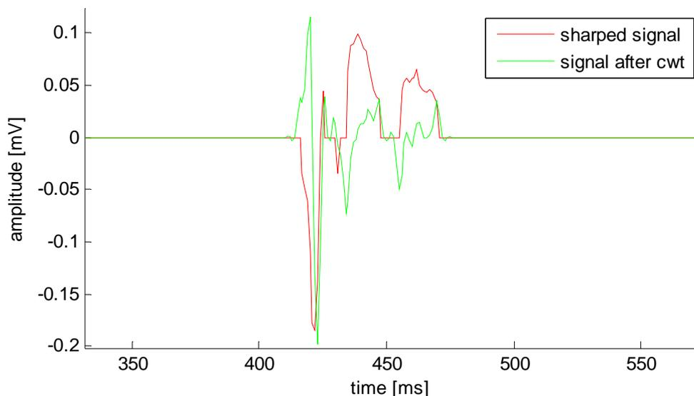
Figure 2: Adjustment signal continuous wavelet transform - CWT, bior1.5. For clarity, only the first pick was detected excitation signal. It is clearer and shows how the signal continuous wavelet transform based on original changed shape.
