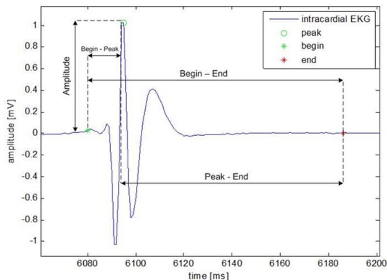
Figure 7: Sample calculations within a single impulse detected
