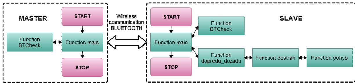
Fig. 4: Relationship between MASTER and SLAVE blocks and their internal structure
