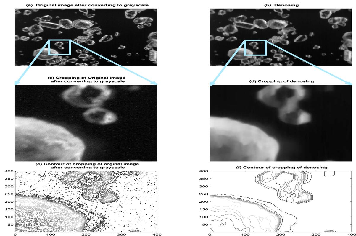
Figure 1: Processing of microscopic crystal image presenting at (a) original image conversion to grayscale image, (b)  $5 \times 5$  median filtering, (c) cropping the grayscale of original image, (d) cropping of grayscale denoising image, (e,f) contour of cropping grayscale original image and contour of cropping grayscale denoising image
