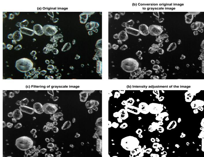
Figure 3: Procedures on (a) microscopic crystal image presenting, (b) conversion of grayscale image and, (c) application  $5 \times 5$  median filtering, (d) presenting suitable intensity adjustment for improvement of segmentation
