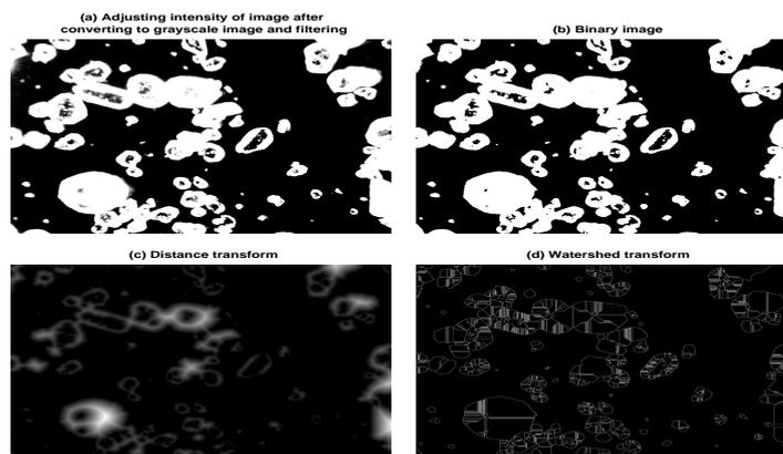
Figure 4: The process of segmentation **(a)** in original image after conversion to grayscale and filtering, **(b)** in binary image followed by, **(c)** distance transform of binary image and, **(d)** final result of watershed transform on microscopic crystal image
