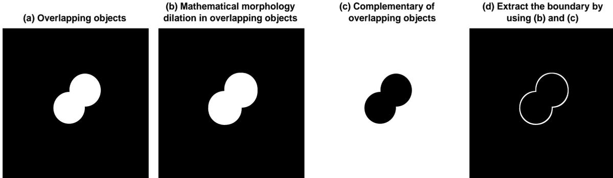
Figure 7: Processing of (a) simulated image (of size 512x512) of overlapping objects, (b) dilation of overlapping objects in a binary image, (c) complementary of overlapping objects, (d) final result for extraction boundary of overlapping objects by using dilation and complementary of image
