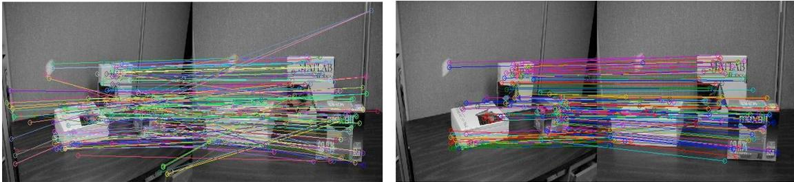
Figure 4: Image correspondences before and after use algorithm for elimination false correspondences (picture is taken from [15]).
