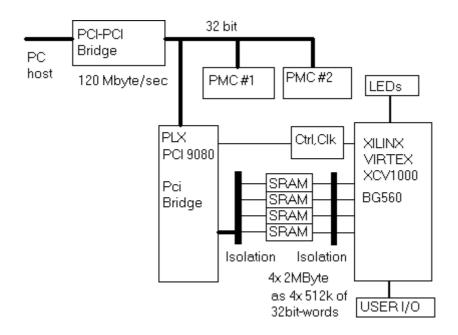
Fig. 5: block diagram of the RC1000 board [11].
