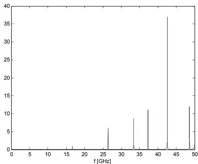
**Fig. 4: Frequency spectrum for square waveguide, 20 cells per side**
