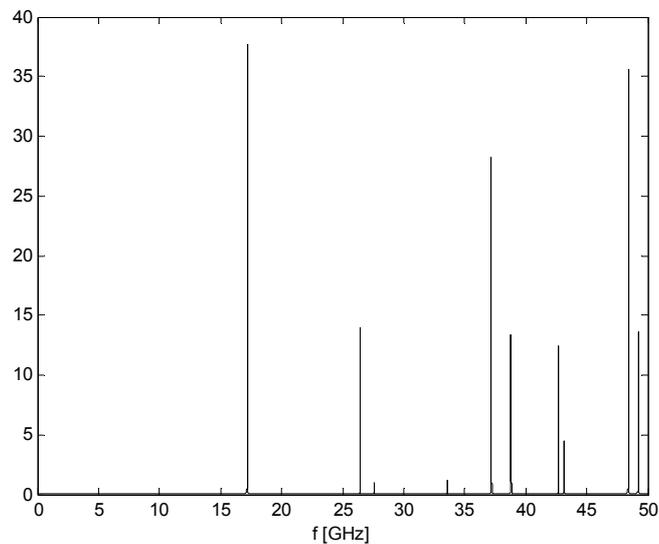
**Fig. 5: Frequency spectrum for shielded air-strip line, 20 cells per side**
