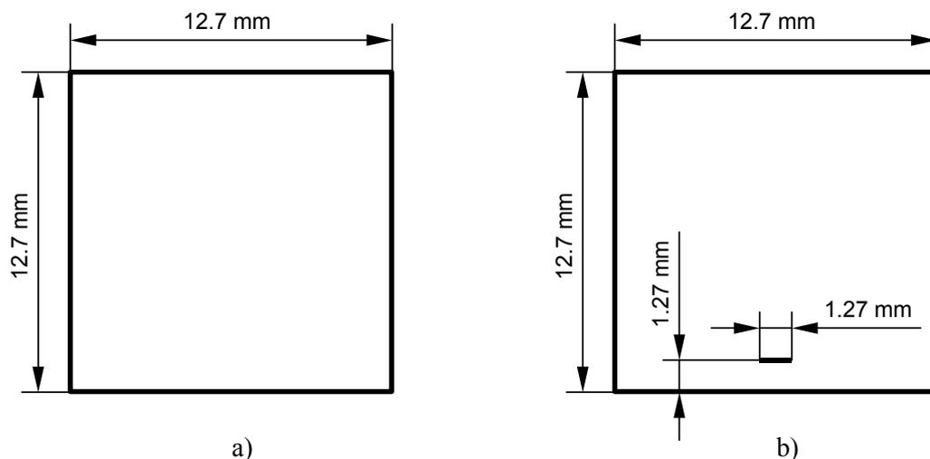
**Fig. 3: Cross sections of analyzed types of transmission lines:**
