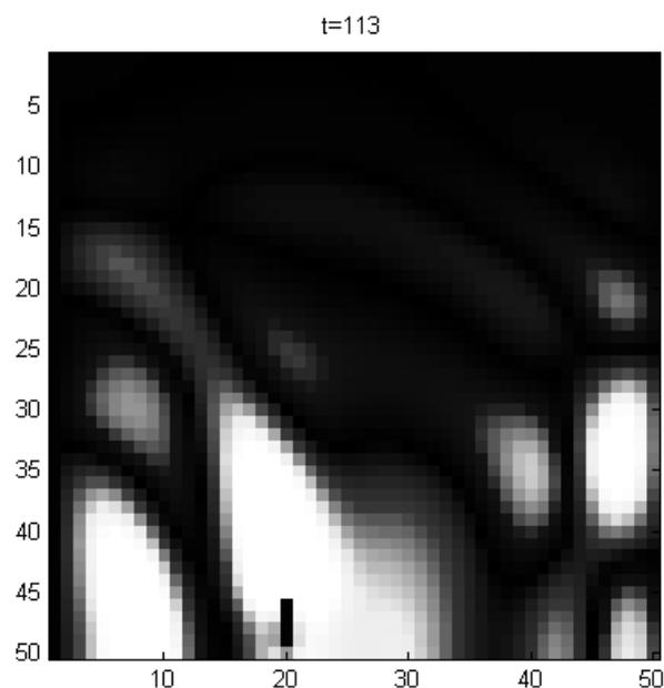
**Fig. 2:** The  $E_z$  field component in cavity resonator after 113 time steps
