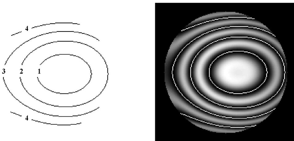
**Fig.6:** Process of numbering of interference fringes (closed fringes)
