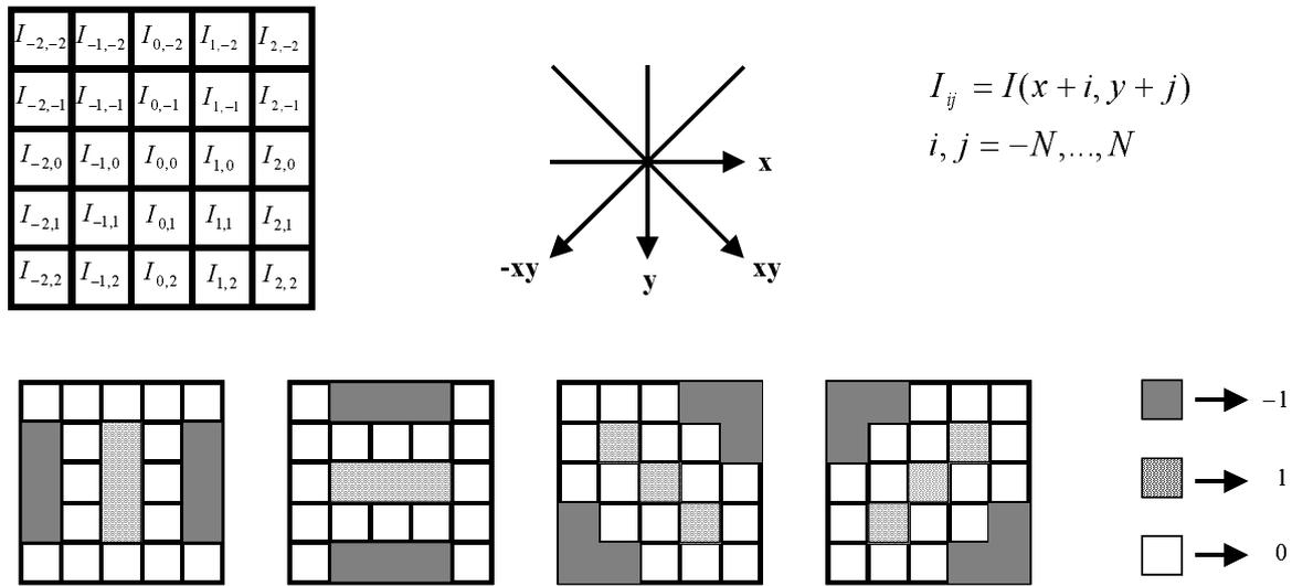
**Fig.3:** Scheme of the operator for an automatic identification of fringe centres
