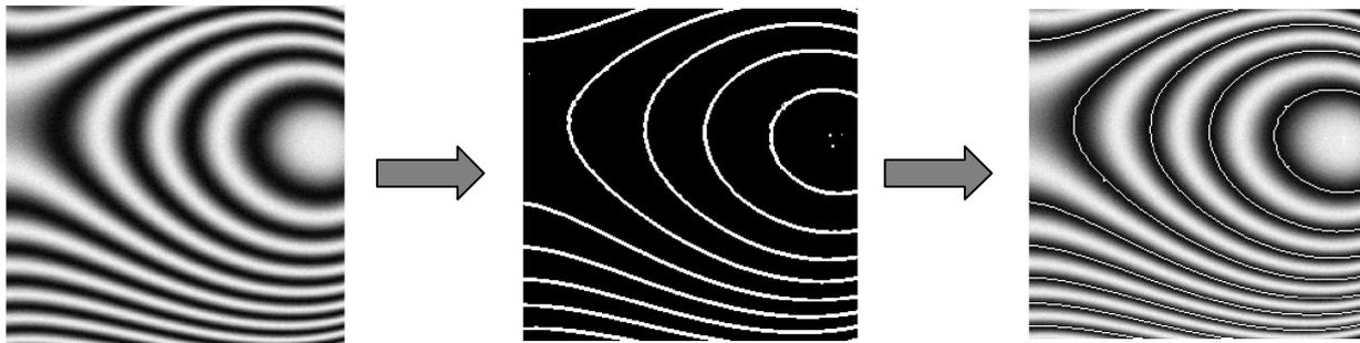
**Fig.4:** Process of automatic identification of fringe centres
