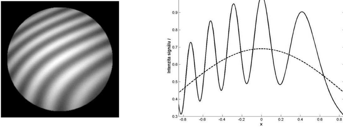
**Fig.1:** Interferogram with the cross-section of the interference pattern
