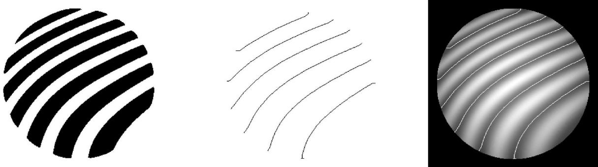
**Fig.2:** Segmentation of the interference pattern
