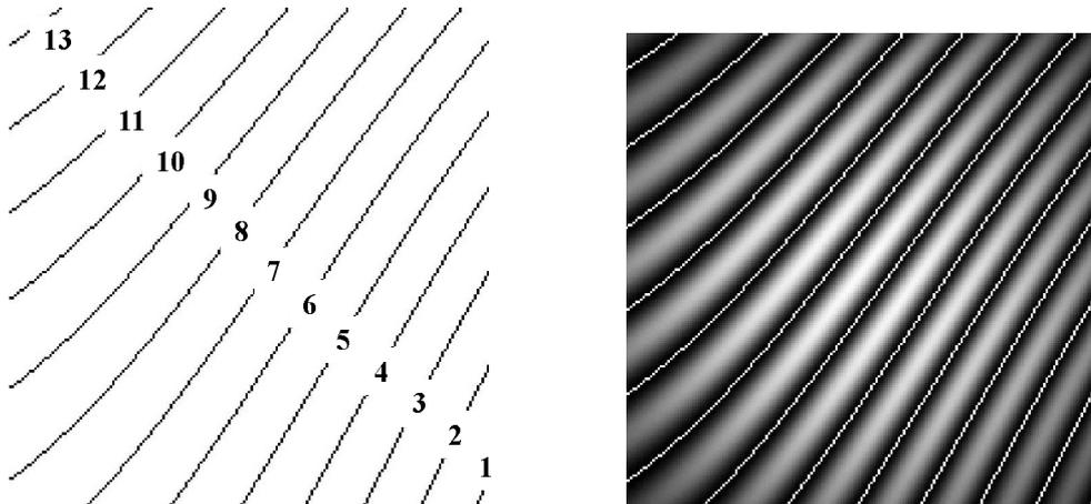
**Fig.5:** Process of numbering of interference fringes (open fringes)
