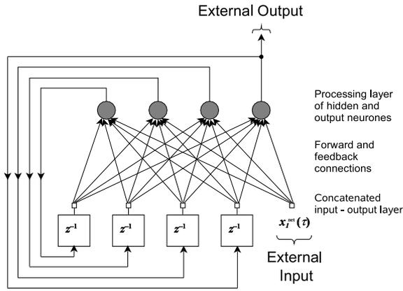
Figure 3: Architecture of recurrent network with one external input and one output [4]
