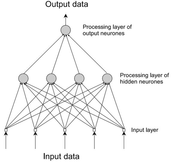
Figure 2: Architecture of two layer feed forward network
