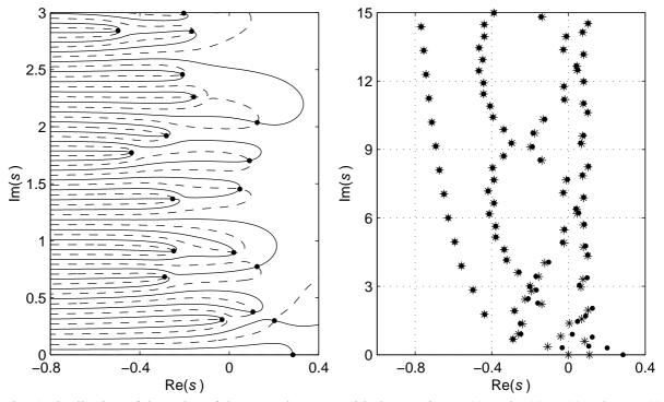
Fig. 6 Distribution of the poles of the neutral system with the matrices  $\mathbf{A}(s)$  and  $\mathbf{D}(s)=\mathbf{A}(s)$ , where  $\mathbf{A}(s)$  given by (22), left part -  $R(\beta,\omega) = 0$  (solid),  $I(\beta,\omega) = 0$  (dashed) right part - distribution of the poles on enlarged region  $\mathfrak{D}$ , dots - spectrum of
