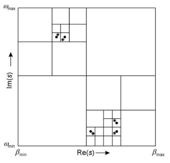
Fig. 3 Locating the roots by Weyl's algorithm asterisks - quasipolynomial roots, black dots - approximations of the roots
