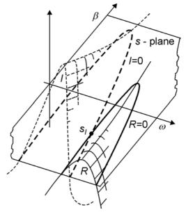
Fig. 4 The principle of locating M(s) roots  $R=\operatorname{Re}(M)=0$  - solid,  $I=\operatorname{Im}(M)=0$  - dashed
