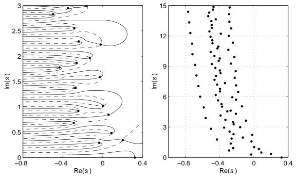
Fig. 5 Distribution of the poles of the retarded system with matrix  $\mathbf{A}(s)$  given by (22). left part -  $R(\beta, \omega) = 0$  (solid),  $I(\beta, \omega) = 0$  (dashed) right part - distribution of the poles in the enlarged region  $\mathfrak{D}$
