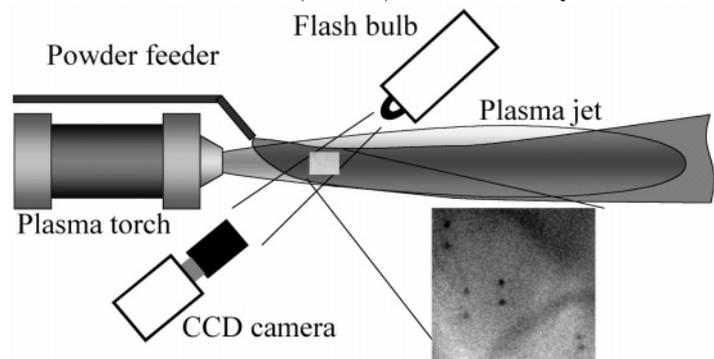
Fig. 1. Experimental arrangement. Axis of the CCD camera and the flashbulb is perpendicular to sheet
