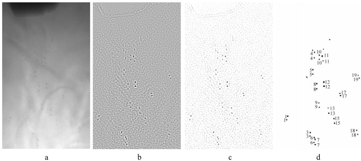
Fig. 3 Part of example photo before filtering (a), after (b,c) filtering, and with marked particles(d)
