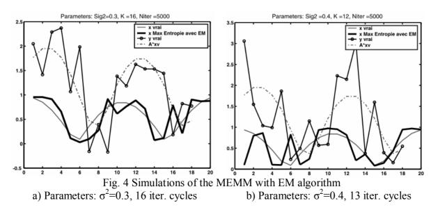
The noise and its distribution can lead to the reconstruction faults that can cause the estimated signal distortion. In this case, the Monte Carlo analysis is applied to avoid the method mistakes and computing faults. It allows to reconstruct the estimation  $\hat{x}$  of the real signal x from measured, very noisy observations y with high precision.
