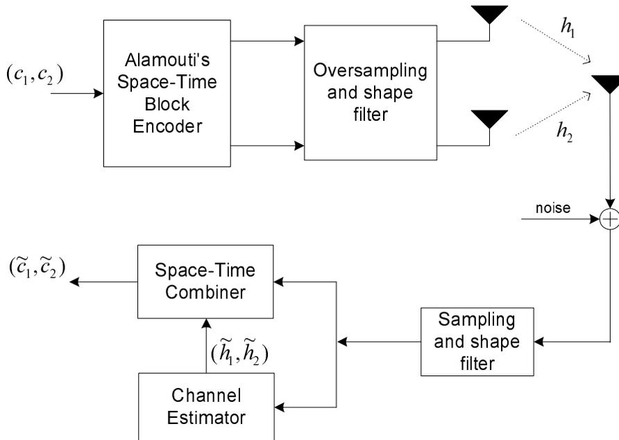
Fig. 2: Discrete-time baseband diagram of the space-time system.
