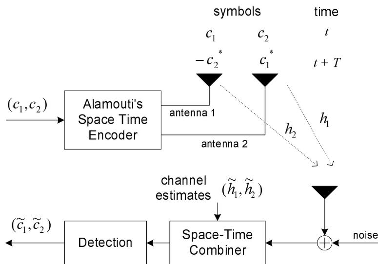
Fig. 1: Alamouti's two antenna transmit diversity scheme.
