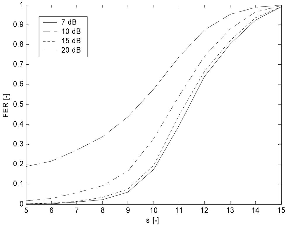
Fig. 3: FER performance vs. frequency selectivity
