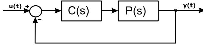
Figure 1: Closed control loop
