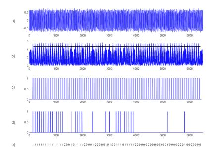
*Fig. 1.* 3*PSK demodulation a) original 3PSK signal, b) correlation level and threshold, c) set of windows, d) binary signal, e) decoded data*
