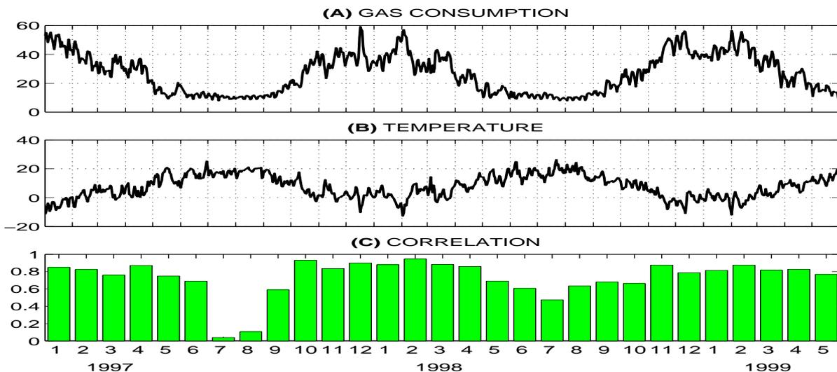
Figure 3: Correlation between temperature and gas consumption (months)
