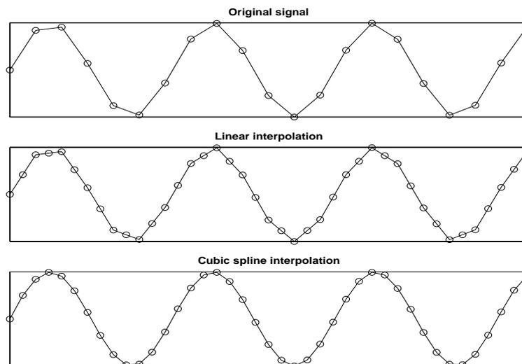
Figure 4: Linear and spline interpolation
