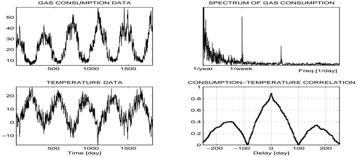
Figure 2: (a) Gas consumption data (b) Spectrum of gas consumption (c) Temperature data (d) Correlation between temperature and gas consumption
