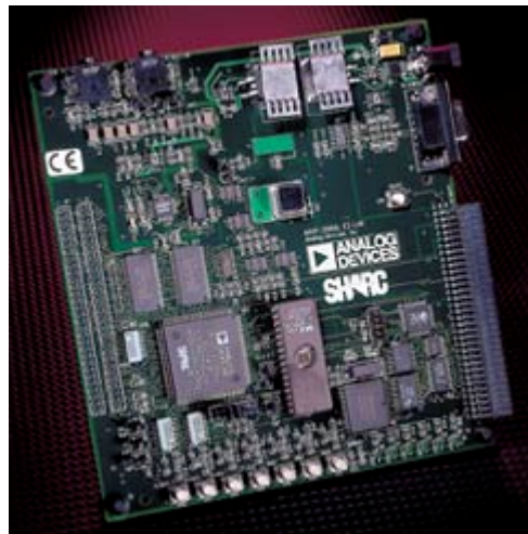
Figure 1: EZ-KIT Lite with ADSP-21065L SHARC DSP
