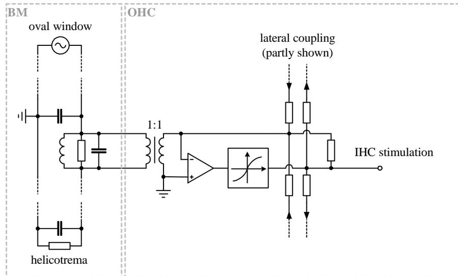
Figure 3: One section of the cochlear model. Basilar membrane and OHC circuits outlined.
