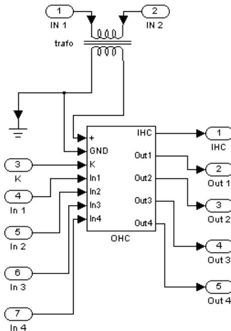
Figure 8: A single OHC circuit.
