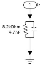
Figure 11: The terminating impedance.
