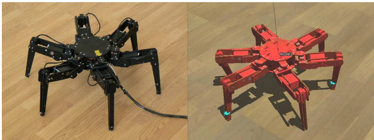
Figure 6: Six-leg walking robot prototype and its virtual model
