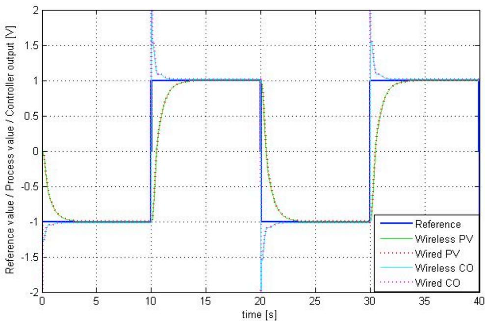
Figure 9: Wired and wireless NCS simulation results
