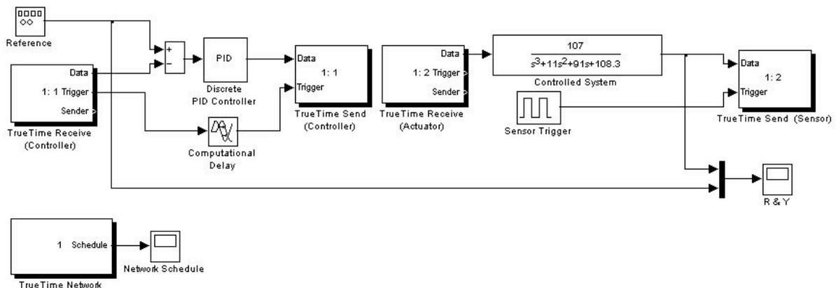
Figure 7: Wired NCS simulation model with standalone interface blocks
