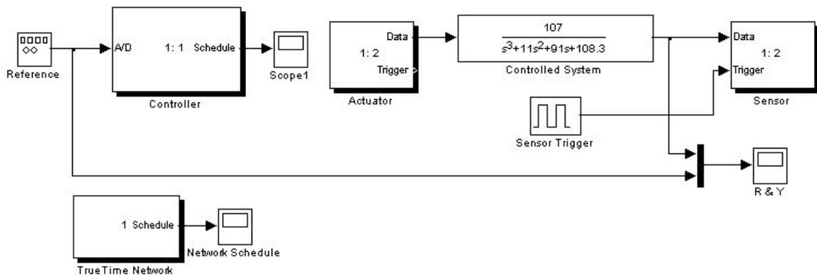
Figure 11: Wired NCS with a kernel block and standalone blocks
