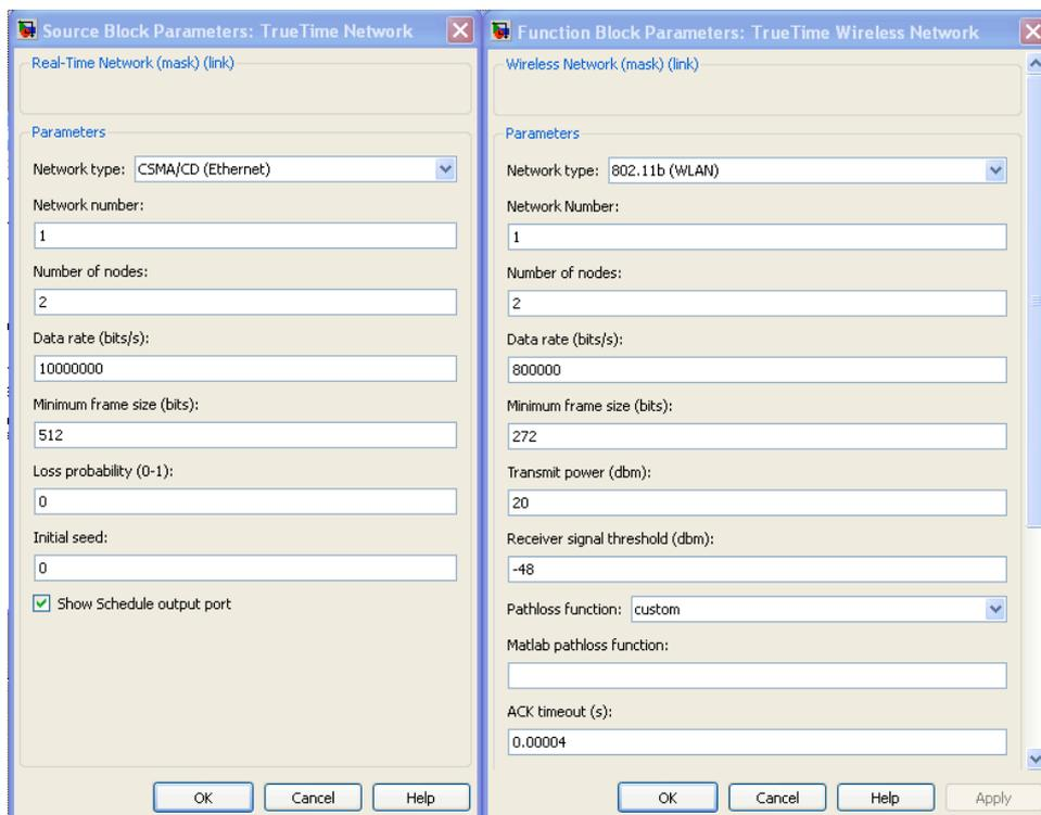
Figure 4: The TrueTime Wired and Wireless Network block masks
