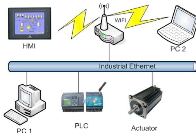
Figure 1: The bottom level of the company's manufacturing process (Hybrid NCS)
