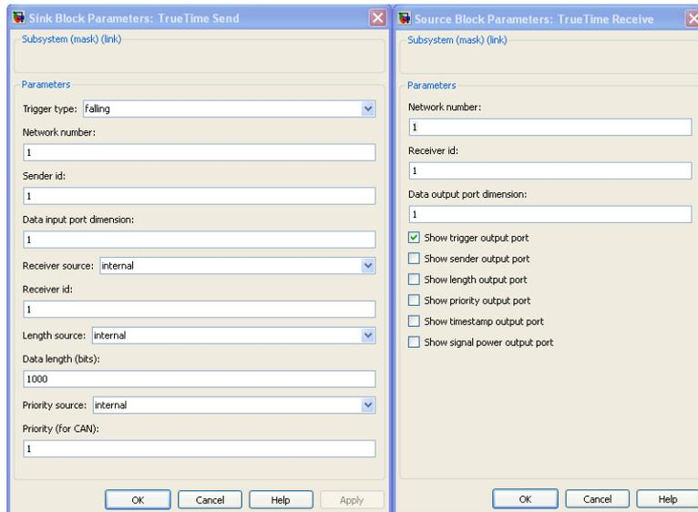
Figure 6: The TrueTime Send and Receive block masks
