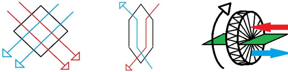
Figure 2: Examples of three types of recuperation units. From right: crossflow, counterflow and rotational
