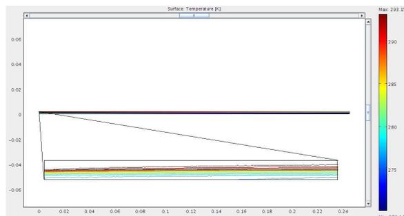
*Figure 5: Heat zone described in color scale by Surface feature and threshold temperatures described by Isosurface feature in case of outer air temperature as 0°C (273 K)*
