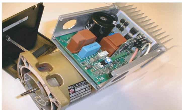
Figure 2: Two-phase drive using voltage inverter and 3-phase low-cost motor [3]
