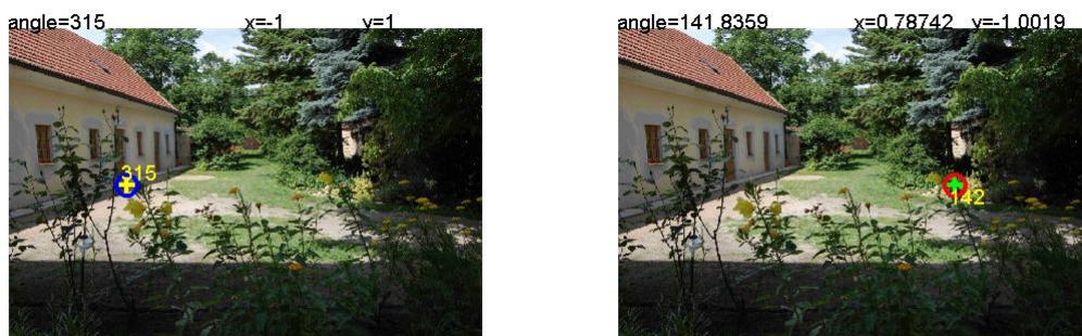
Figure 2: Examples of the operator's interface. The position of the joystick is marked by the cross, the blue color means, that operator points in front of the user, red color means behind the user.
