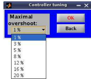
Figure 16: Choice of the maximal overshoot using analytical Naslin method
