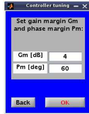
Figure 18: Parameter setting using analytical method based on gain and phase margin
