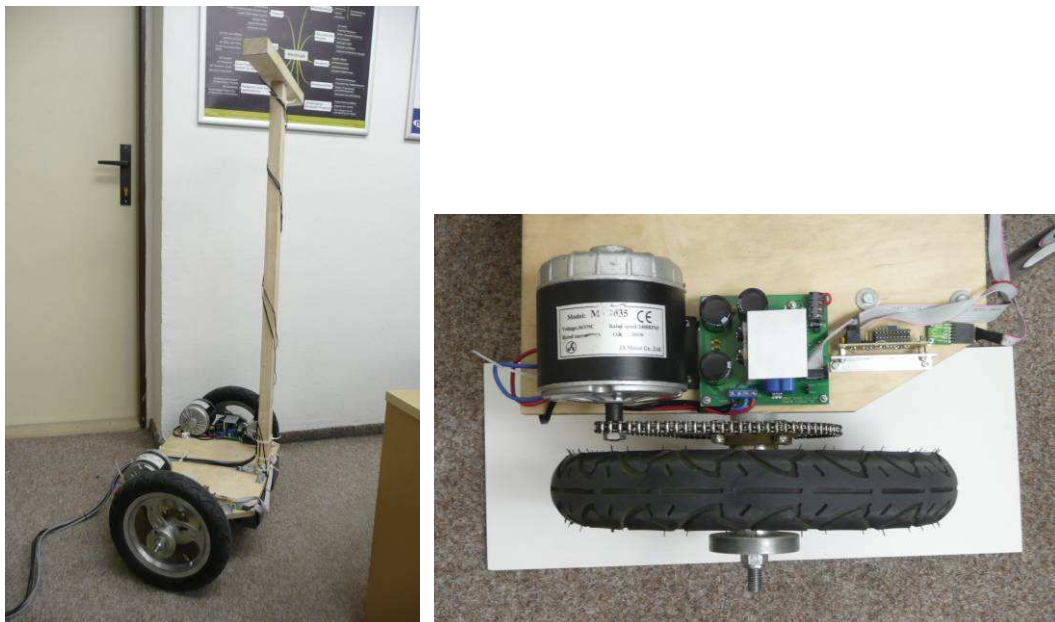
Figure 2: Self-balancing H1 controlled using MF624 and Real-Time Toolbox directly from Simulink (left); Detail of DC motor, H-bridge and gyro (right)
