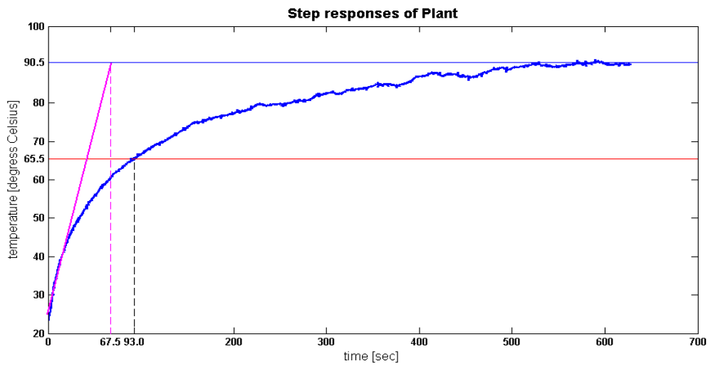
Figure 4: Identification from step response
